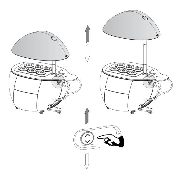
The direction of the arrow on the button indicates the direction of the dome actuation.
